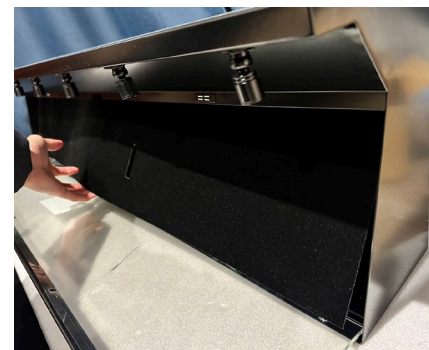
③ Carefully remove the backboard to avoid scratching the acrylic panel.
