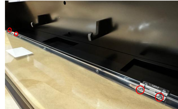
Remove the four screws securing the panel to the hinges, then remove the acrylic panel.
