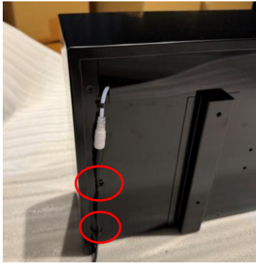
Connect the supplied AC cable and always secure it with the clamp.
