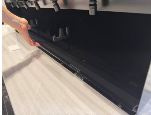
Remove the base (magnetically attached). ※ Be careful not to crush the velour.
