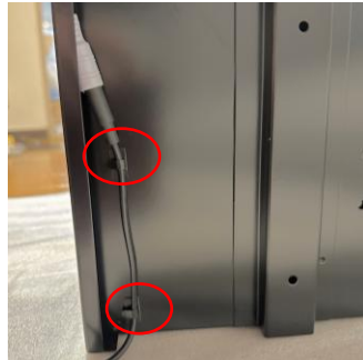
Fasten the AC line with a clamp.
